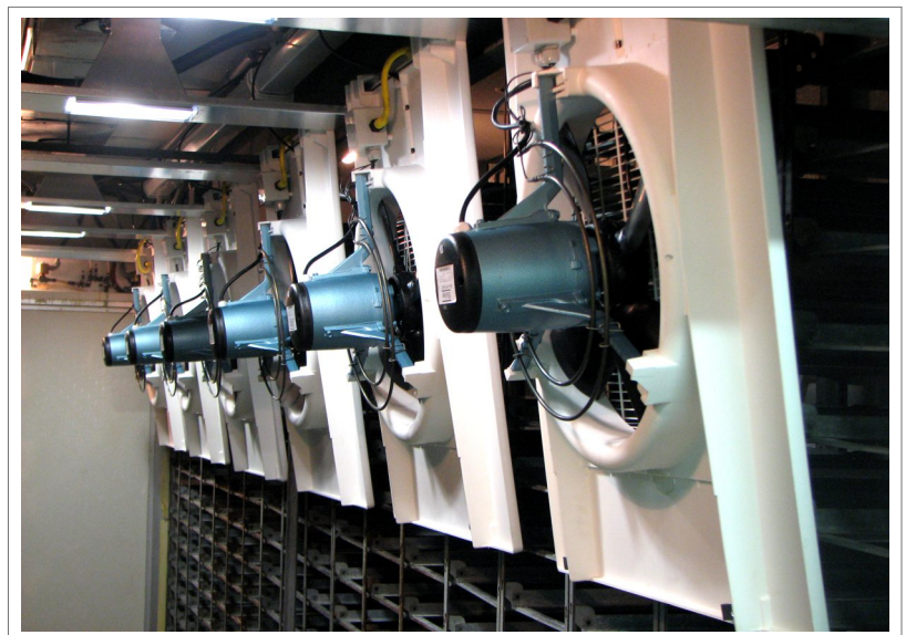
Ring heating element and cyclomist humidity system mounted to plastic fan board assembly
