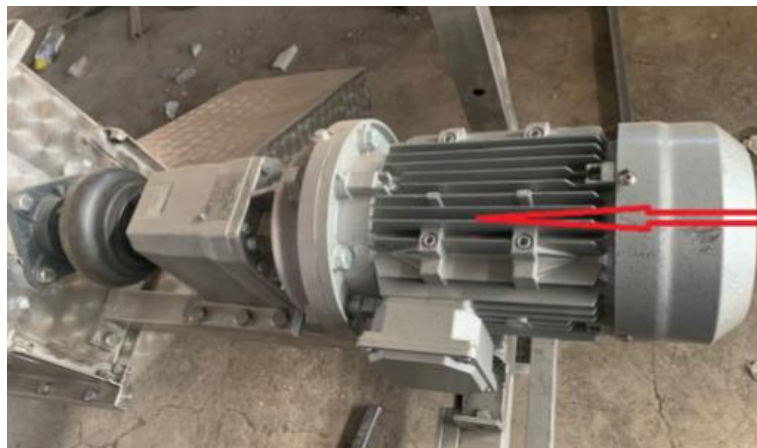
MOTOR 2.2KW 400V 3 PHASE WITH INLINE GEAR BOX AND OUTPUT SHAFT
